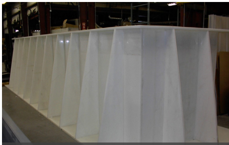
All plastic vertical buttress tank
