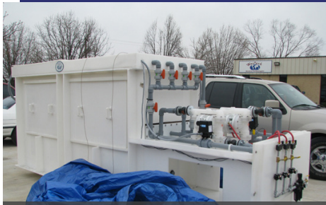
Flux tank filtering vessel
