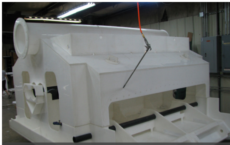
Steel strip pickling tank and hood
